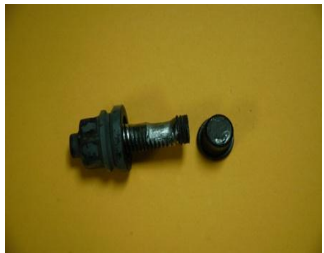
Figure 2: Extreme wear on lug
