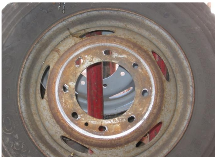
Figure 1: Notice elongated lug holes
